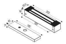
**WMG600** Lock: 8" x 1<sup>23</sup>/<sub>32</sub>" x 1<sup>9</sup>/<sub>16</sub>" (203mm x 43.5mm x 40mm)
