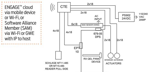
**Operation:** Presenting a valid credential to Schlage MT XX-485 will cause QEL panic device to retract for authorized entrance and enable exterior actuator. Free non-alarmed egress at all times. Interior actuator always active to retract QEL panic and open door.
